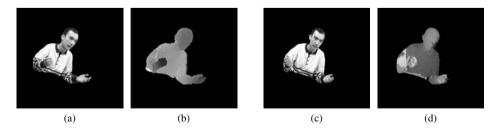
Figure 7.5 Matching results with hybrid recursive matching: (a) left; (b) left disparity; (c) right; (d) right disparity
