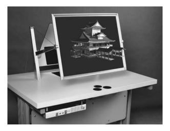
**Figure 14.12** Prototype free-viewing VAMR display. The display creates high-resolution aerial 3D images which float 25 cm in front of the screen (filter panel) within the user's arm reach. A video-based hand tracker is embedded in the desktop at a location corresponding with the aerial image
