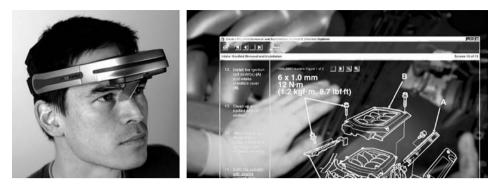
**Figure 14.1** By superimposing test and repair data into vision, the Nomad Augmented Vision System allows reading detailed service information and following complex instructions directly at the point of task (Reproduced by permission of Microvision Incorporated)
