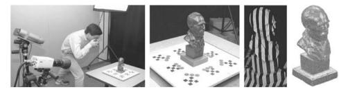
**Figure 4.11** Data acquisiton process (Reproduced by permission of the ACM from Chen *et al.* 2002): (a) capturing many images; (b) sample image; (c) painted object; (d) 3D triangular mesh
