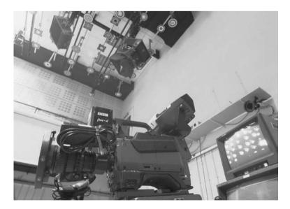
**Figure 3.1** The BBC 'Free-D' camera tracking system is based on circular bar-coded targets on the ceiling and an auxiliary camera looking upwards. Real-time hardware computes the position and orientation of the camera at a 50 Hz update rate
