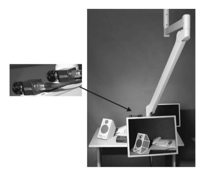
**Figure 14.15** Articulated video-MMR system. The monitor mounted on the arm can be freely moved within a large working envelope, while it shows the scene captured with stereo cameras. Information about the target object (a loudspeaker) is superimposed in correct perspective onto the live scene (in this example the wireframe). The system enables a natural real-time user interaction
