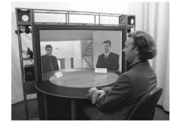
**Figure 11.10** Immersive virtual environment video conference setup at Fraunhofer HHI, Berlin. In this scenario persons from different remote locations are arranged around a virtual table. Each participant can be compressed as an arbitrarily shaped video object using the MPEG-4 object-based coding modes (Tanger *et al.* 2004)
