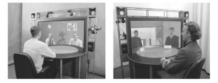
**Figure 5.12** Semi-immersive videoconferencing on its way to the market. *Left*: the experimental system of the European IST project VIRTUE using a 61-inch plasma display. *Right*: the immersive meeting point (im.point), a follow-up prototype of VIRTUE using a MPEG-4-based software implementation and standard PC technology
