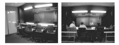
**Figure 5.13** The RealMeet room system. *Left*: the system mounting with two screens connected to two different remote sites. Each screen uses a semi-transparent mirror, like the Telepresence Wall from figure 5.4 *Right*: a running session with one remote site connected. Reproduced by permission of France Telecom RD
