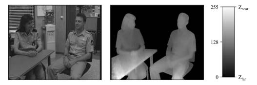
**Figure 2.3** The ATTEST data representation format consisting of: (1) regular 2D colour video in digital TV format; (2) accompanying 8-bit depth-images with the same spatio-temporal resolution
