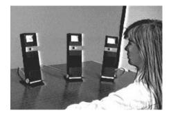
**Figure 5.6** The Hydra concept: a local user is sitting in front of three Hydra units, substituting the remote conferees physically. Each unit consists of its own camera, monitor and loudspeaker. Reproduced by permission of William Buxton (Snellen and Buxton 1992)
